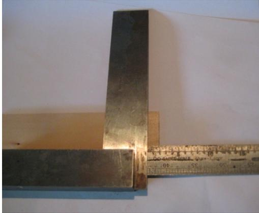
A method least recommended would be to measure down both sides of the board and mark with a pencil. The chance of error is very great as pencil marks are notoriously fat.
